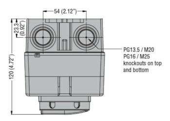
IEC/EN TYPE IP65 NON-METALLIC ENCLOSURE SWITCH DISCONNECTOR, THREE-POLE. WITH ROTATING BLACK HANDLE, 25A
