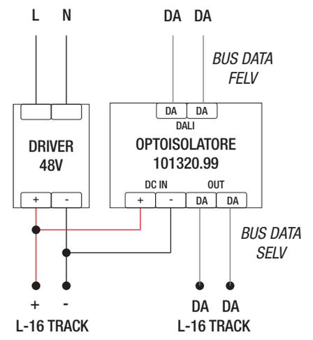
SCHEMI DI CABLAGGIO L-16 TRACK + L-16 EVO CON STRIPLED WHITE 24Vdc O 48Vdc
