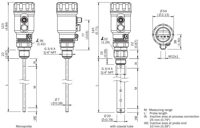
IAE: Inactive area at probe end 10 mm (0.39")
