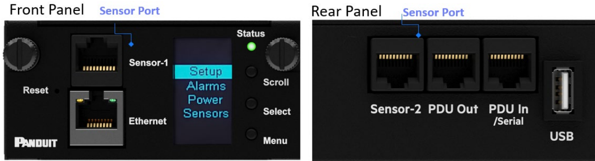
Figure 84: Sensor Ports for Horizontal PDU
