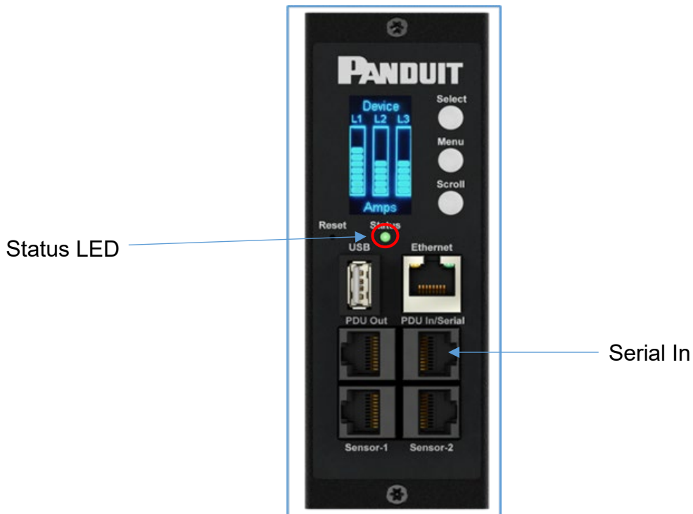
Figure 2: Status LED & Serial In Port Identified
