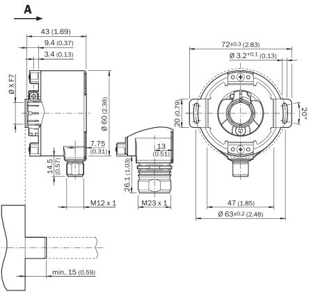
General tolerances according to DIN ISO 2768-mk Cable diameter = 5.6 mm +/- 0.2 mm bend radius = 30 mm
