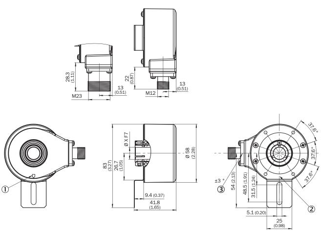
XF7 values see shaft diameter table for through hollow shaft, clamping at the back
