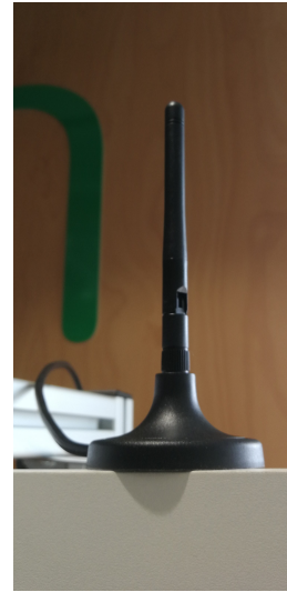
Module antenna outside the cabinet
