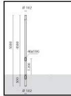
S.2814 POTEAU CYLINDRIQUE H 4,5m Ø102mm
