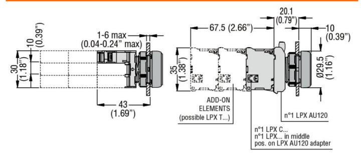
LED INTEGRATED LAMP-HOLDER, STEADY LIGHT PLATINUM SERIES, SCREW TERMINATION, 12...30VAC/DC. WHITE
