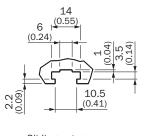
Sliding nut groove for side mounting
