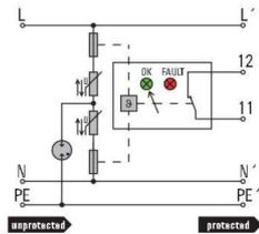
Schematic circuit diagram
