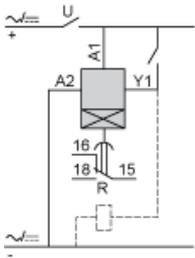
Function A : Power on Delay Relay
