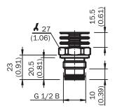
Housing with L-connector (DIN EN 175301-803 A)
