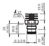
Housing with L-connector (DIN EN 175301-803 A)
