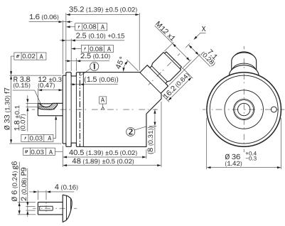
Non-tolerated dimensions according to DIN-ISO 2768-mk
