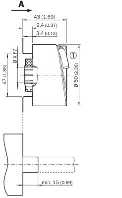
General tolerances according to DIN ISO 2768-mk (1) Cable diameter = 5.6 mm +/- 0.2 mm bend radius = 30 mm
