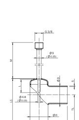
Protection tube with process connenection
