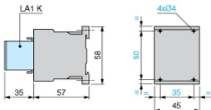
Contactors LC1 K, LP1 K, LP4 K: Mounting on Rail AM1 DP200 or AM1 DE200 (35 mm)
