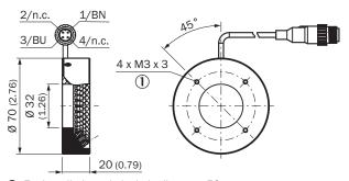
1 For installation; pitch circle diameter 50 mm
