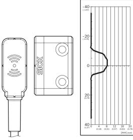
Safe switch on distance  $S_{ao}\,6~\text{mm}$
