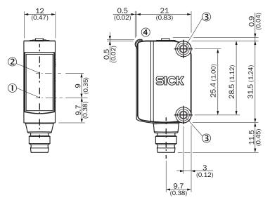
① Center of optical axis, sender
