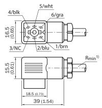
(1) Minimum bend radius at dynamic use  $R_{min}$  = 20 x cable diameter
