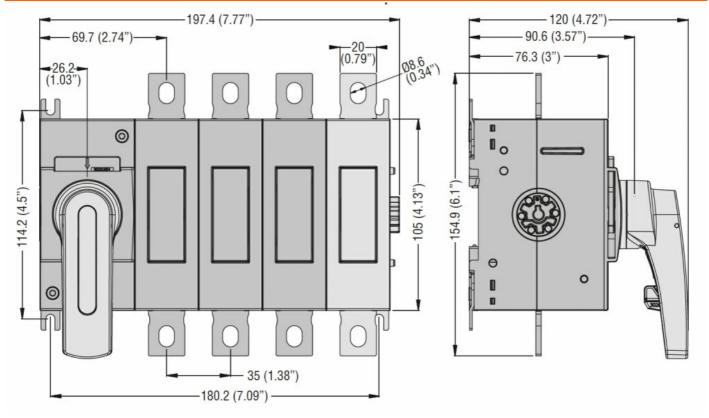
FOURTH POLE ADD-ON, SIMULTANEOUS CLOSING OPERATION AS SWITCH DISCONNECTOR POLES, IEC/EN. FOR GL0160C1...GL0315C1 VERSIONS
