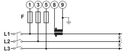
Fig. 12 AV5, AV6 balanced load
