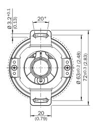
General tolerances according to DIN ISO 2768-mk  $\odot$  Cable diameter = 5.6 mm +/- 0.2 mm bend radius = 30 mm
