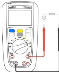
MTX 204 rango \mu\text{A}
