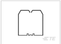
Wiring Duct Product Type: Wire Retainer
