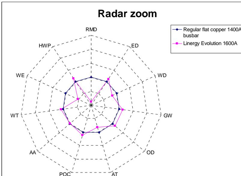
Energy depletion (ED): energy depletion is higher of 15% for Linergy Evolution 1600A compare to regular flat copper busbar 1400A.
