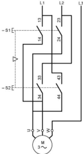
Combined with 3-pole isolating block XACS399 or XACS3991, shown in the unoperated position (pendant station "supplied"), fitted with key release trigger action latching Emergency stop operator.
