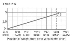
① Maximum contact force when the counterweight is positioned at the end of the rod (260 mm)
