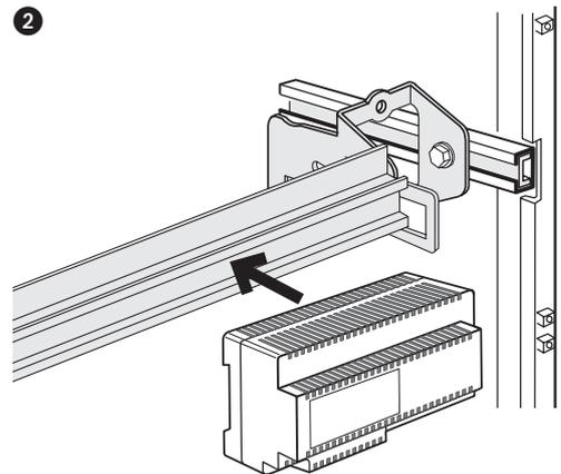
Install the power supply inside of the electrical cabinet.
