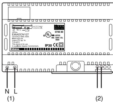
Connect the 127 V a.c. power cables to the terminals (1) and the BUS to the terminals (2).
