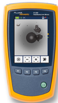
FI-500 displaying a dirty fiber endface
