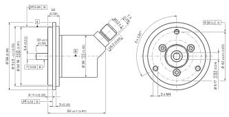
Order example for 6 mm shaft diameter: AHx36I-S3xx0xxxxx + BEF-FA-020-050-I (adapter is not pre-assembled)
