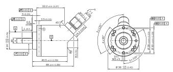
Non-tolerated dimensions according to DIN-ISO 2768-mk
