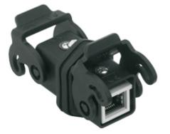
Female RJ45 connector, CYG couplers series, size "21.21", in insulating enclosure, 8 data contacts + 2 power contacts
