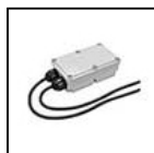
S.2493 Signal converter from DALI to VIRTUAL MIDNIGHT IP67 Compact control module for automatic power reduction / brightness reduction for night-time. The device has an integrated bus supply (20mA) that allows to control up to 7 DALI luminaires / DALI control gear. 2 operating modes are supported: - Operating mode B1: power reduction through mains phase or control phase; - Operating mode B2: power reduction using virtual midnight calculation. All necessary settings can be made using rotary and slide switches present on the device present inside the waterbox. The device must be located before the DALI luminaire / DALI control gear.
