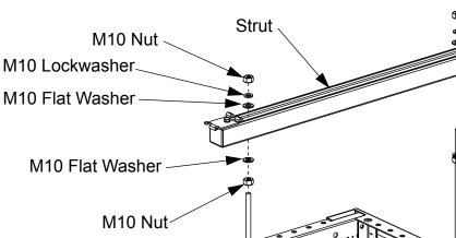
Step 3: Attach Strut to top of Threaded Rods using (1) M10 Flat Washer, (1) M10 Lock Washer, & (1) M10 Hex Nut (per side). Bracket load rating is 300 lbs. maximum. (Torque all M10 Nuts to a maximum of 7 lb-ft. (9.5 N-m) typical)
