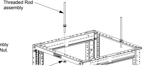
Step 2: Install Threaded Rod assembly in thru holes & secure with (1) M10 Nut.
