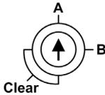
Use only the small, plastic screwdriver provided with the CPU to set the rotary switch according to its role in a Hot Standby system.
