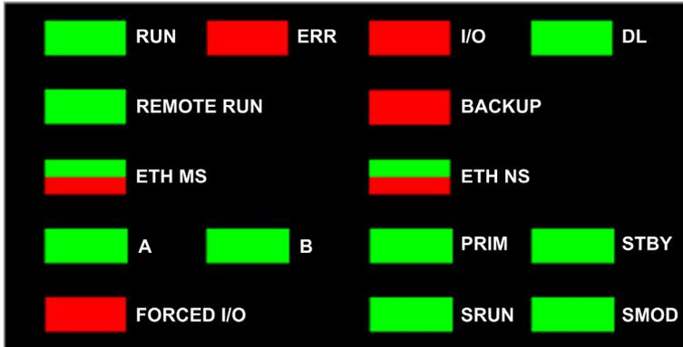
**NOTE:** The **SRUN** and **SMOD** LEDs apply only to safety CPUs.
