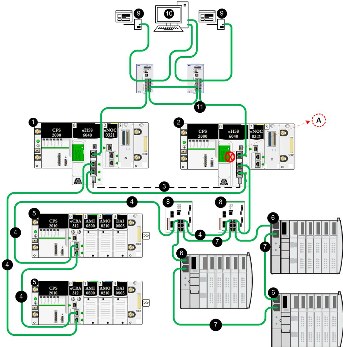
**A** In this topology, where SCADA is connected to the Hot Standby system via the primary and standby CPU service ports, confirm that you select the **Automatic blocking of service port on Standby CPU** check box in the **ServicePort** configuration tab to help avoid network communication loss (formed by cables 4 and 11).
