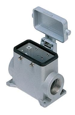
Surface mounting housing, C-TYPE series, with 4 pegs, Pg29 cable entry, size "57.27", high construction, with metal cover
