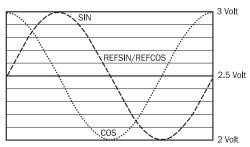
Signal diagram for clockwise rotation of the shaft looking in direction "A" (see dimensional drawing)1 period =  $360^{\circ}$ :  $1024^{\circ}$  Signal diagram for clockwise rotation of the shaft looking in direction "A" (see dimensional drawing)1 period =  $360^{\circ}$ :  $1024^{\circ}$
