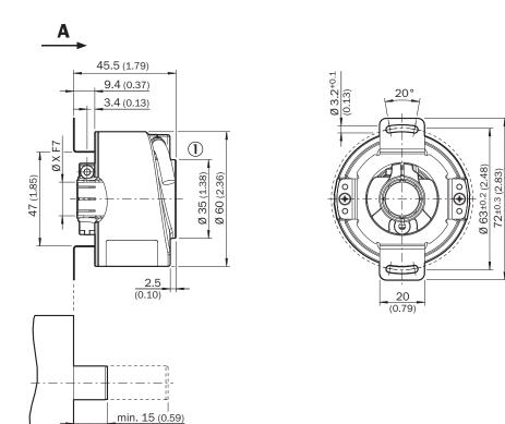
General tolerances according to DIN ISO 2768-mk (1) Cable diameter = 5.6 mm +/- 0.2 mm bend radius = 30 mm
