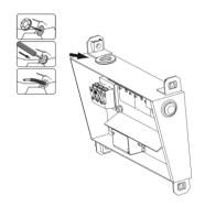
In order to ensure the luminaire is sealed, it is vital to use the cable grommets.
