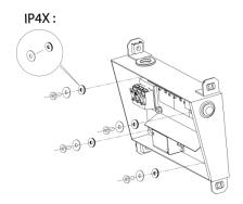
For mounting the luminaire, use 5 mm diameter flatheaded screws with fixing plugs suitable for the type of wall, in order to achieve optimum rip-out resistance. The screws and plugs are not supplied with the luminaire.
