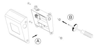
Refit the frame + diffuser assembly using a suitable screwdriver fitted with the 98000004 special bit.
