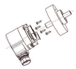
The mounting of the bearing block is performed using the threaded holes machined in the flange or with the help of a flange adapter or angled mounting bracket.
