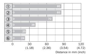
Max. sensing range S<sub>n</sub>, flush or non-flush installation, non-magnetizable material
