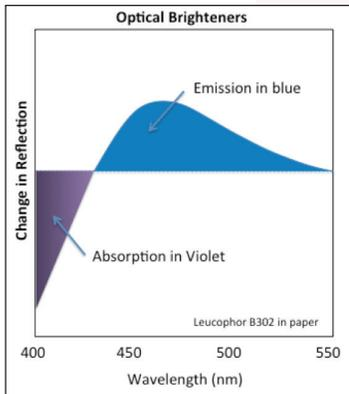
Figure C (above): How optical brighteners work.
