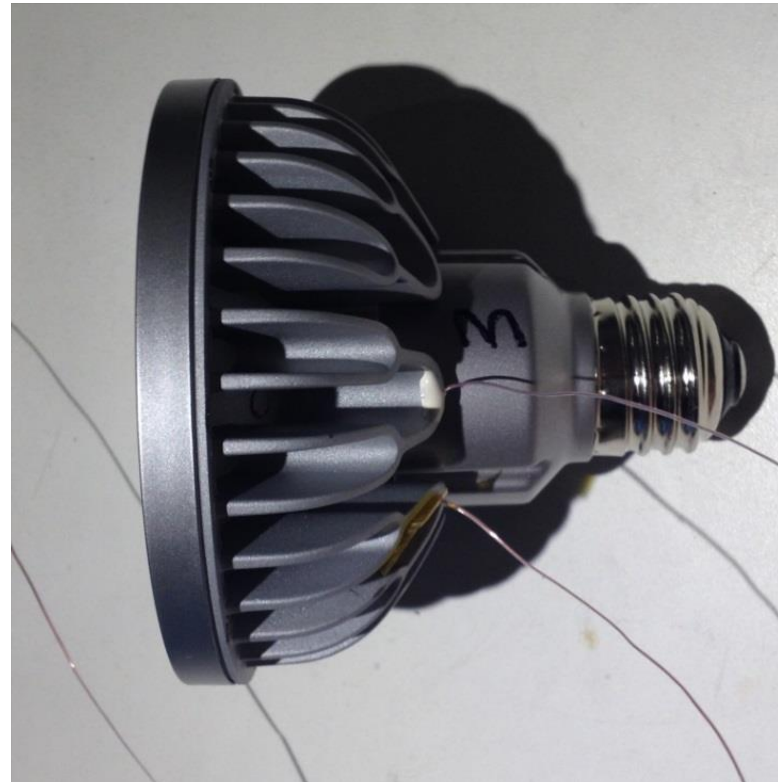
[2]: Thermocouple mounting on a PAR30 lamp.
