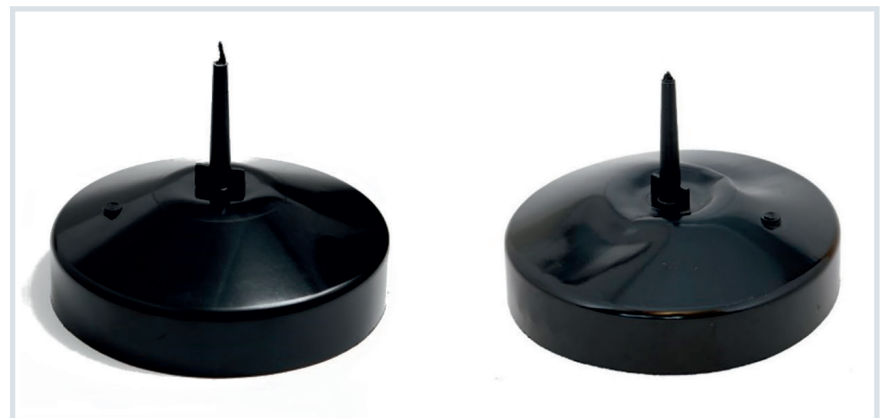
Fig. 4. Molded part, after sufficiently long cooling time (left) and inadequate cooling time (right)
