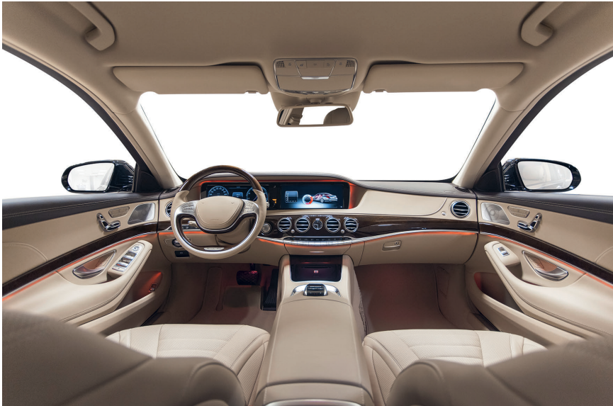
Fig. 3. A new ABS Novodur grade with high heat resistance and impact strength was developed especially for the requirements in the upper interior automotive trim (© Ineos Styrolution)
