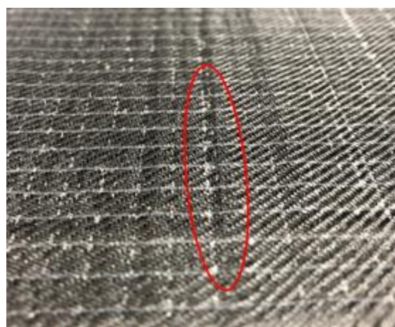
Figure 14: Bubbles on the top ply of the 2 nd generation composite (bubbles encircled red)
