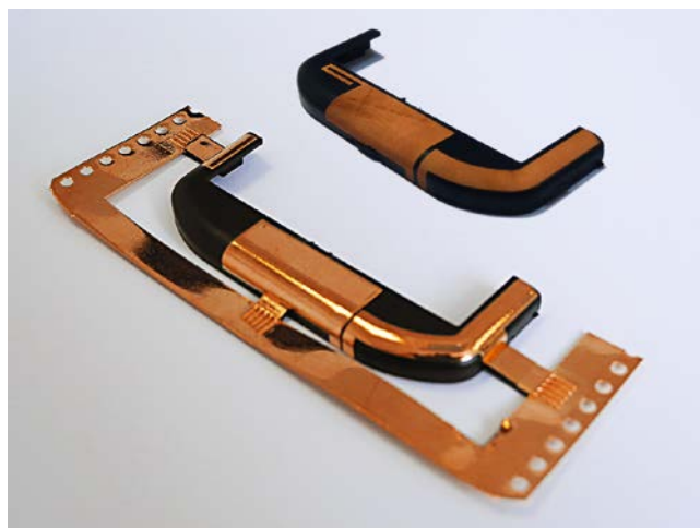
Fig. 4. Front: an antenna with contacts for galvanic reinforcement. Rear: the part with purely chemical copper structure
