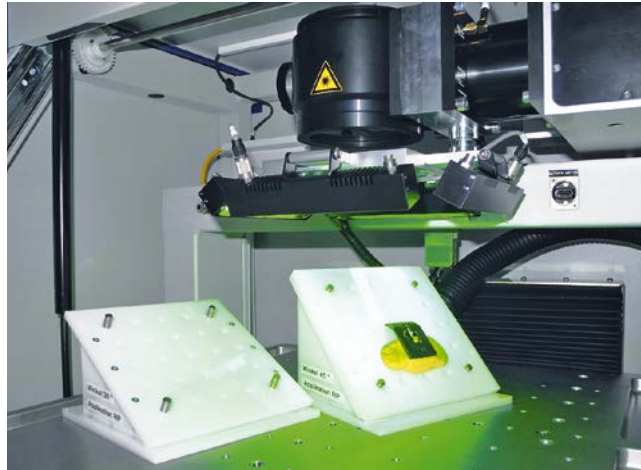
Fig. 2. Simple part holders are adequate for reliable feeding of the LDS parts in the ProtoLaser 3D
